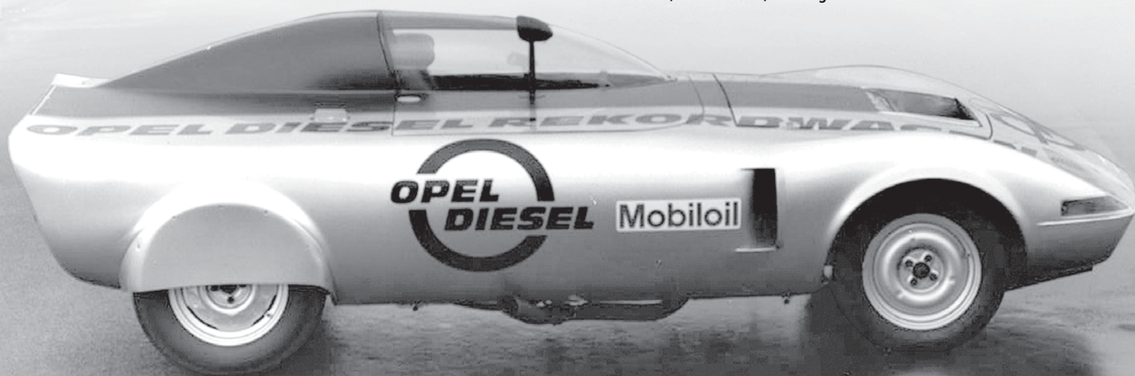
Much of the production Opel GT remained in the record-holding car: the chassis, transmission, steering and brakes were all stock
