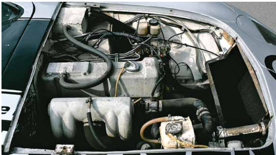
Opel hoped to smash the record with the company's new 2.1-liter, four-cylinder, turbocharged diesel. The engine featured a single overhead cam and two valves per cylinder
