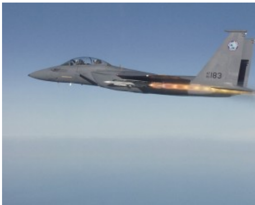
Boeing's Silent Eagle flight demonstrator aircraft fires an AMRAAM from its stealthy weapons bay during flight testing July 14, 2010. Photo courtesy of The Boeing Company
