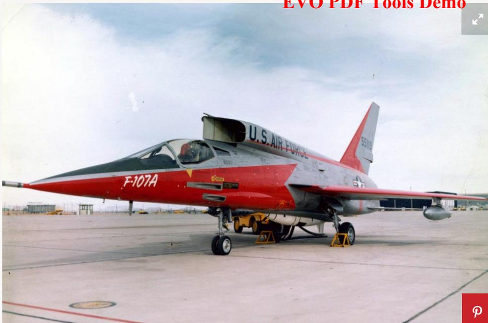
The Air Force's need for a big, nuclear-capable fighter/bomber in the mid-1950s led North American to use its successful [F-100 Super Sabre](#) design as a jumping off point for the new YF-107A. The craft would need a big radar antenna placed in the nose where the F-100 had its intake, so the YF-107's designers placed the intake above and behind the cockpit, giving the airplane its distinctive look and earning it the nickname "man eater."
