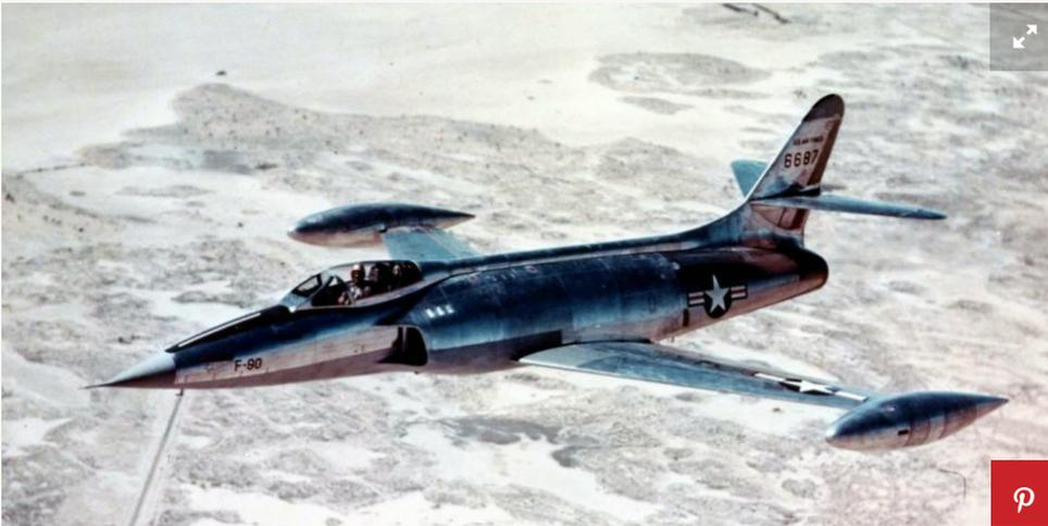
Looking ahead as WWII drew to a close, the Army Air Corps issued a request for a long-range advanced fighter that would be able to escort bombers. Lockheed came up with a design based on its [P-80 Shooting Star](#), but instead of a single engine and straight wing, the XF-90 featured two Westinghouse J34 turbojets— 6,200 lbs total thrust—and 35-degree swept wings. Two prototypes were built, the first flying in June 1949.
