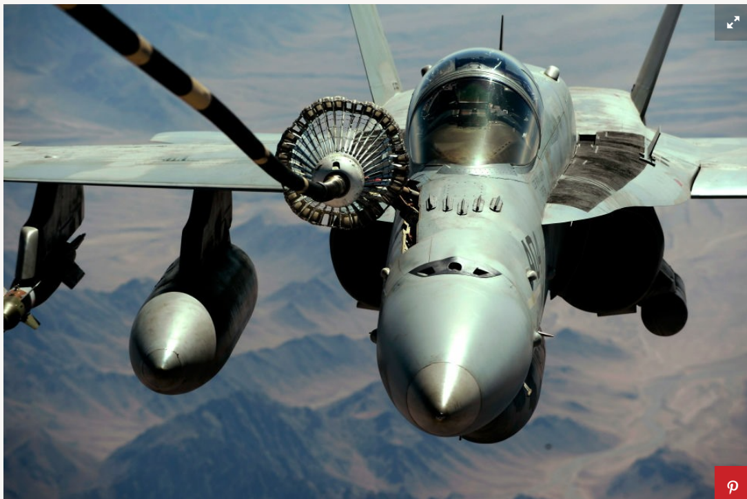
An F/A-18 executes in-flight refueling through an aerial refueling system. The systems are required for all carrier-based tanking missions. (U.S.Navy photo)
