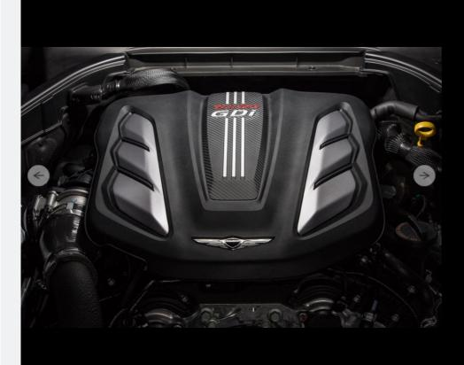
Under the hood is a 3.3L twin-turbo V6 with 365hp.
