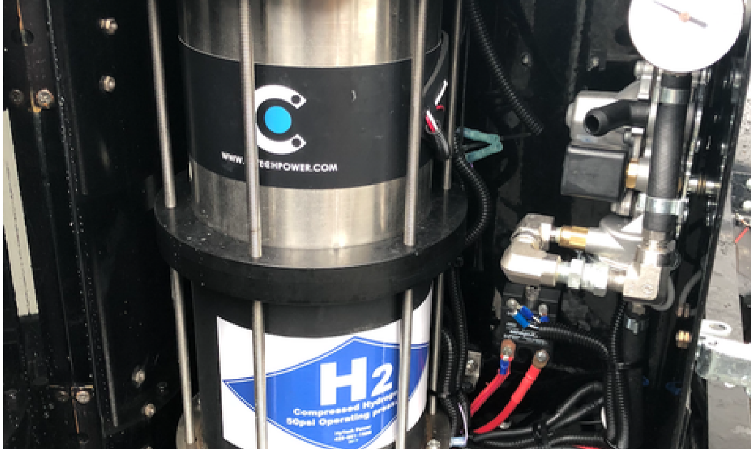
HyTech Power's water tank for electrolysis with patented catalyst inside.
