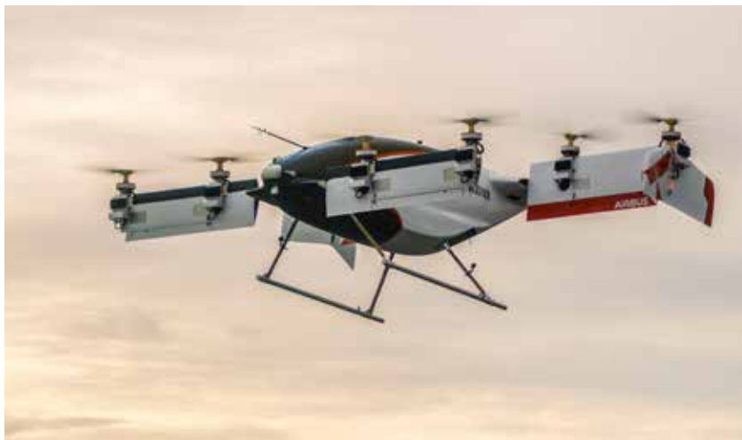
▲ Airbus' single-seat Vahana concept, which had its first full-scale flight test last year. Photo: Airbus
