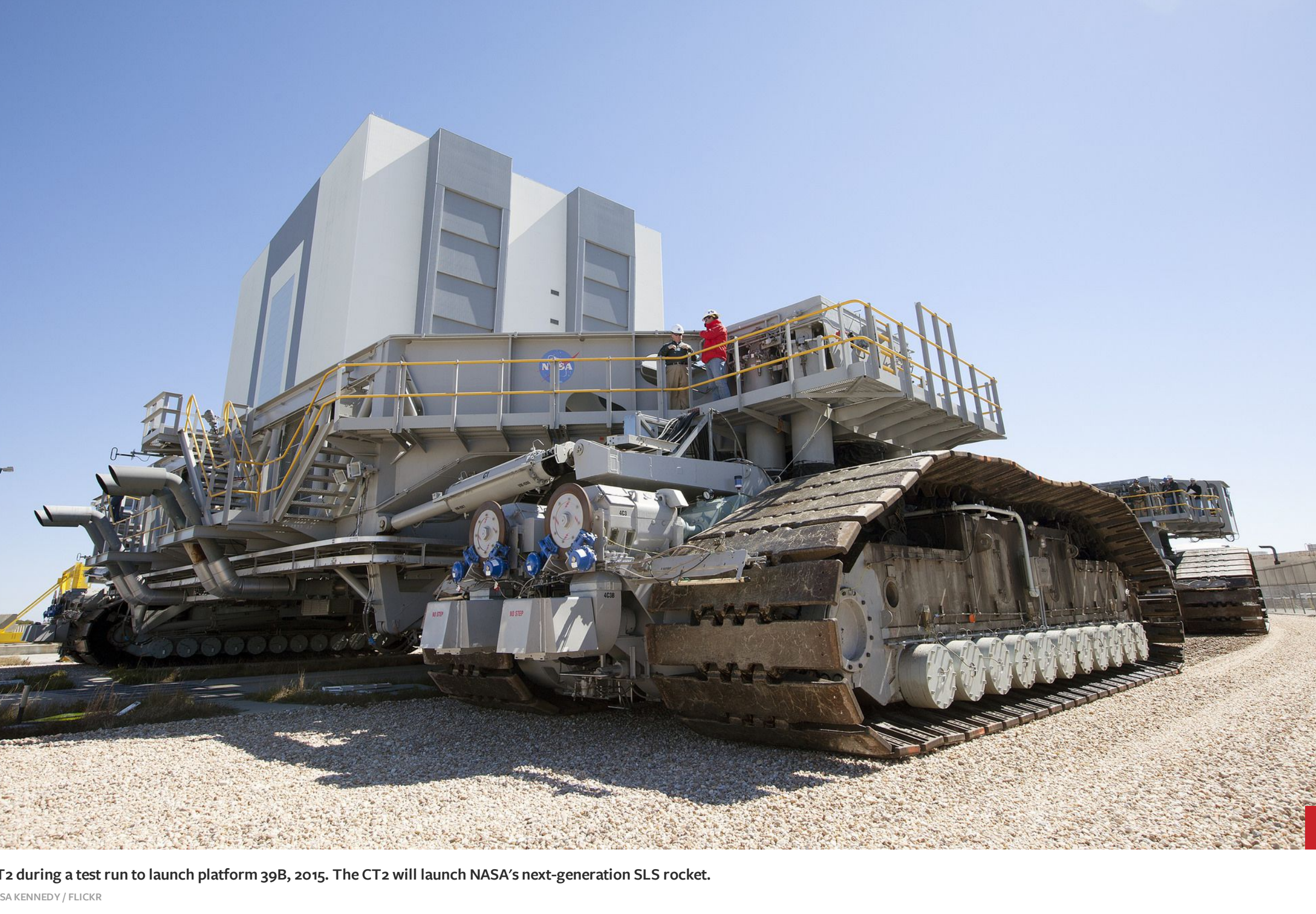
CT-2 during a test run to launch platform 39B, 2015. The CT-2 will launch NASA's next-generation SLS rocket.
