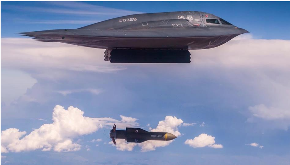
A B-2 Spirit drops one of two GBU-57 Massive Ordnance Penetrator bunker-busting bombs as seen in a... [+] U.S. AIR FORCE
