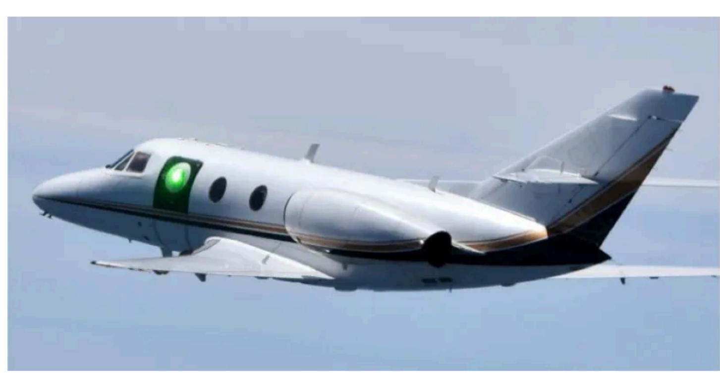
The Dassault Falcon 10 test aircraft carrying the HARDROC beam director illuminated by a low-power laser during test flights in August 2022
