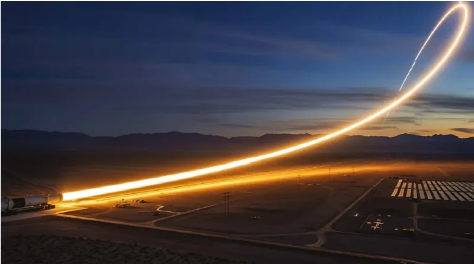
Longshot's accelerators lie flat on the surface rather than standing on a pad, which is what keeps the civil engineering cheap »
